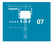
The rigid platen, as well as the cope flask, are aligned within the squeeze station by the zero-clearance linear guiding system. This maintains precise alignment of the drag and cope flasks as the platen raises the drag up to close the flasks. These features combine to eliminate any mold shift as the mold is produced.
