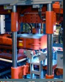
The HLM's sealed linear bearings, motion slides, and magnetic rodless cylinders replace cam followers, wheels, tracks, and rails to provide smoother, quieter, more energy-efficient operation and greater machine stability, with less maintenance required.
