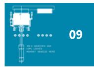
The hopper car is retracted, positioning the squeeze head over the cope flask in preparation of squeeze. With the flasks held in precise alignment, the platen goes up and the mold is squeezed under high pressure.
