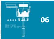
The hopper car is also pushed out to the squeeze station in preparation for filling the cope.
