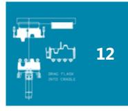
After the drag mold has been lowered, the drag flask is retracted back into the cradle. During coresetting operations the drag flask can now be filled in preparation for the next mold while the squeeze station is available for coreset.
